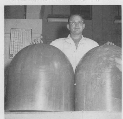
FINISHED DUST COVERS are shown by Richard Olive. After the glass cloth and resin lay-up is completed, the entire mold is covered with a plastic bag and a vacuum created to force the air out.
